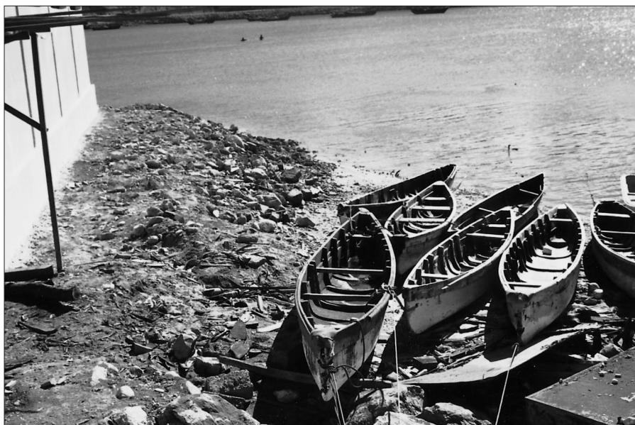
Fishing hūris : the inside of the hull is carved with ribs, Sur, Oman
