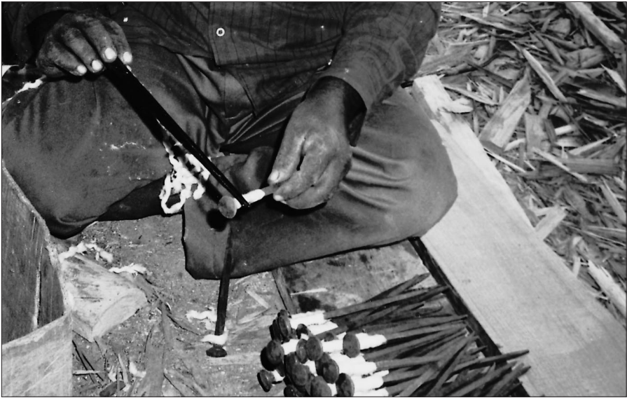
Wrapping nails in oiled fibre
