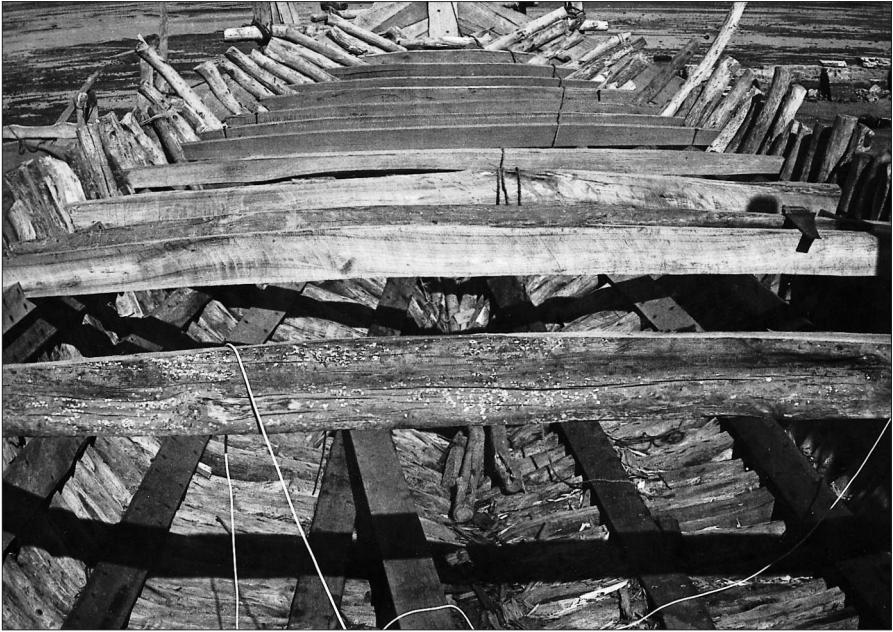
The main ṣuwār (deck beams) are laid on the beam-shelf (photo courtesy of Rainer Hartel)
