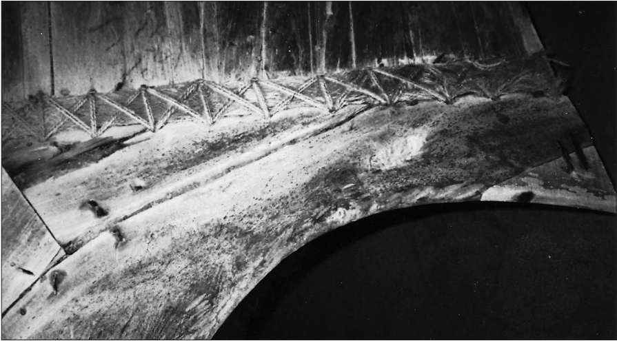
Badan showing the hull planking stitched to the sternpost, Al-Hail near Muscat, Oman
